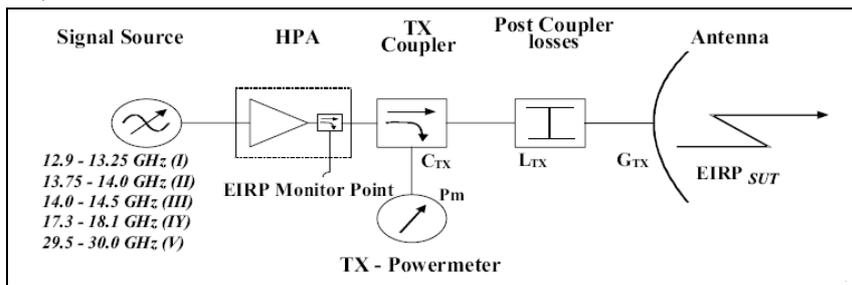
Unless stated otherwise, antenna diagrams will be normalized to typical antenna gain (e.g.: corresponding to 65% efficiency at Ku-Band test frequencies). If applicable, please indicate appropriate reference gain:
