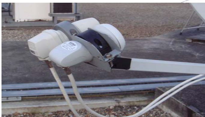
Dual-feed LNB for reception from 9/13°E
