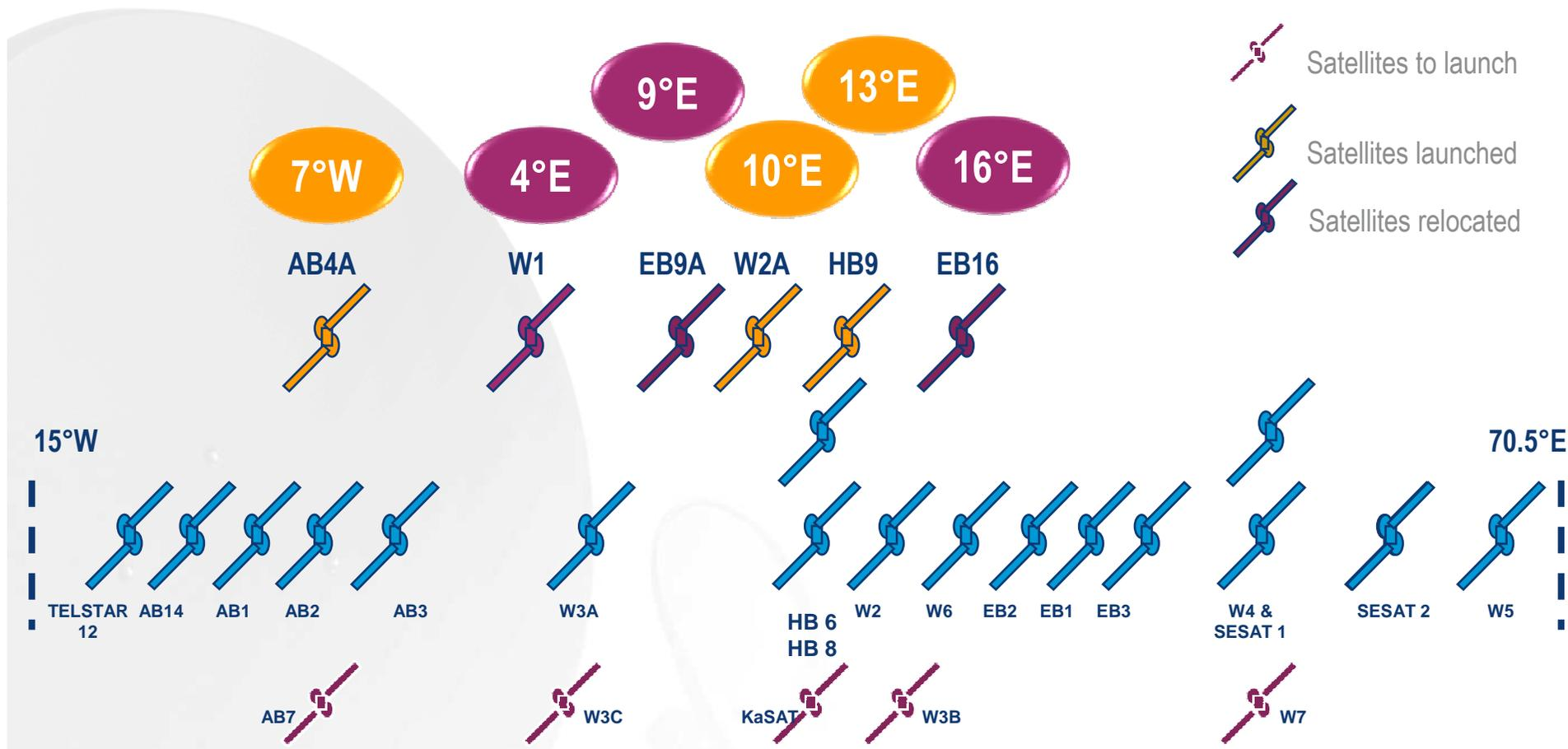
Eurobird 4 and Eurobird 9 are currently drifting . W2M is deployed at 3°E but not in commercial service
