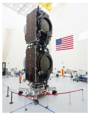
EUTELSAT 115 West B stacked with its co-passenger Photo: Boeing
